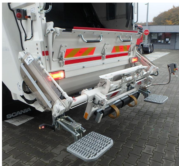
Figure 2. Lifter SK350 – one of the most popular bins lifting system
